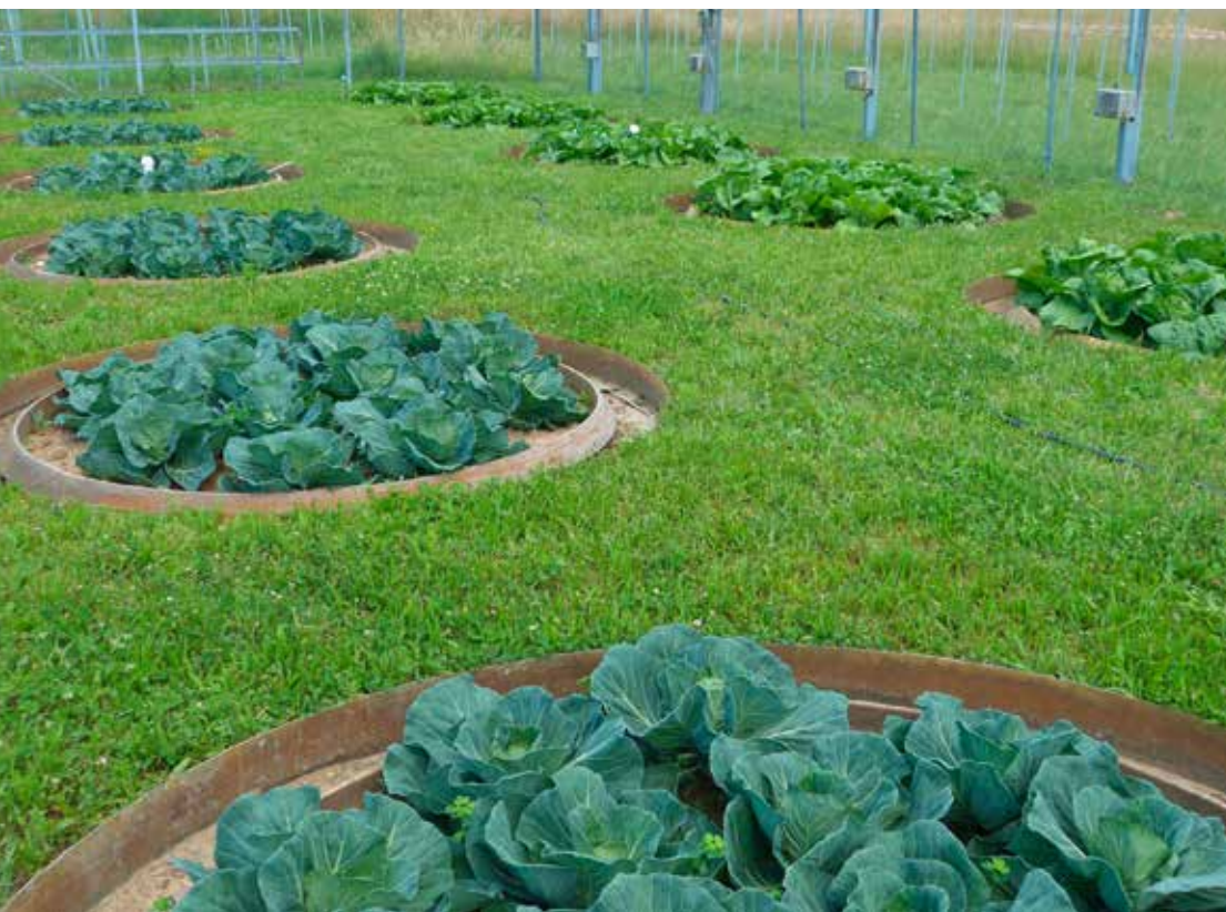
Measuring nitrate leaching under vegetable crops with lysimeters. (Photo: Ernst Spiess, Agroscope)
