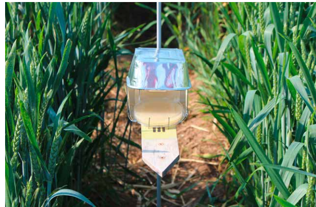
Figure 3 | Spore trap with a Fusarium -selective medium adjusted to the same height as the flowering wheat heads (design: Hans-Rudolf Forrer, Agroscope; photo: Dimitrios Drakopoulos, Agroscope).
